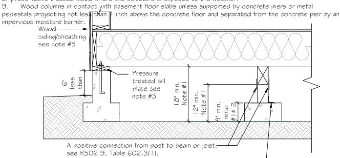
A positive connection is required from footing to the post to prevent lateral displacement at the bottom end of the post or column R407.3
