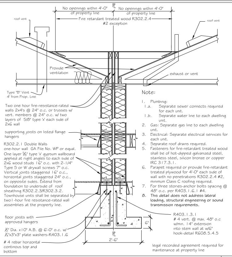
Trusses and joist perpendicular to wall of townhouse Two-One Hour
