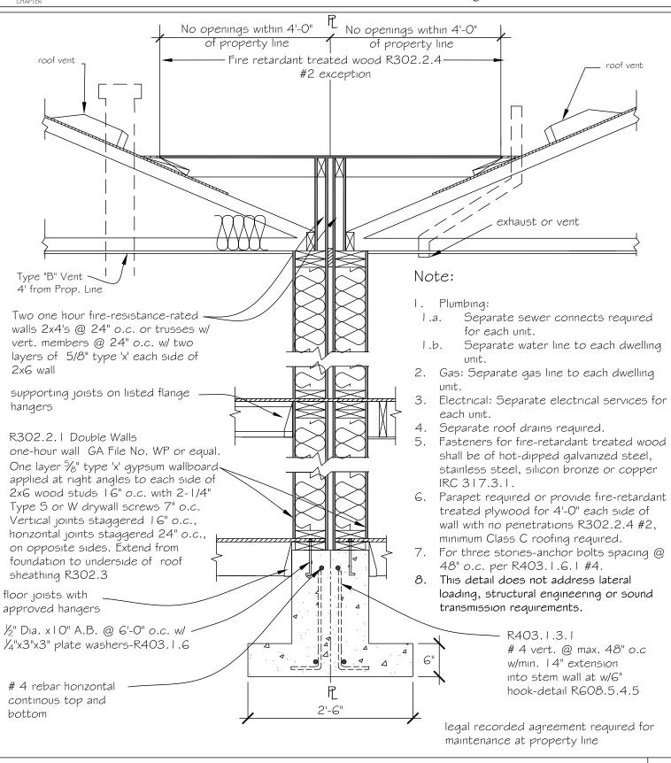
Trusses and joist perpendicular to wall of townhouse Two-One Hour
